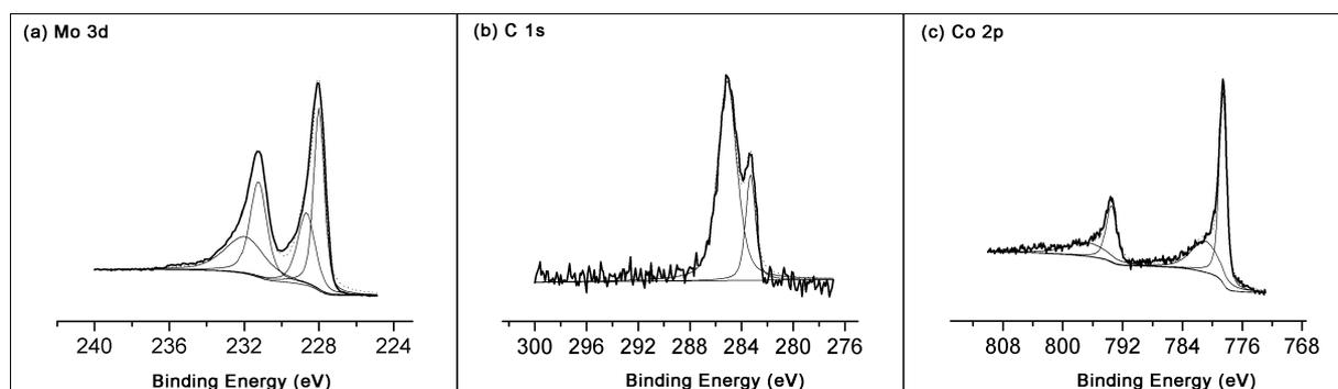
**Fig. 6** XPS spectra of Mo 3d (a), C 1s (b) and Co 2p (c) of  $\text{Co}_3\text{Mo}_3\text{C}$ . Thick curves represent the raw data, thin curves represent the results of deconvolution of the spectrum into Lorentzian-broadened Gaussian peaks, and dotted curves represent the resulting fit to the raw data.
