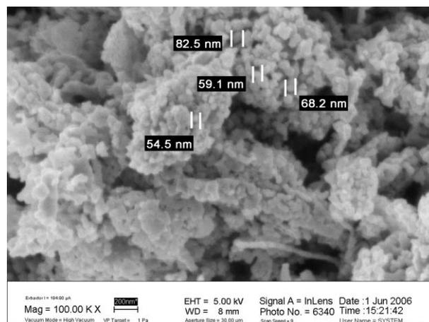
Fig. 4 SEM image of as-prepared  $\text{Co}_3\text{Mo}_3\text{C}$ .
