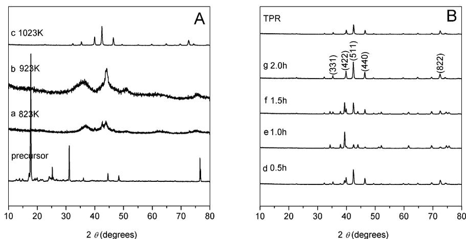
Fig. 1 XRD patterns of  $\text{Co}_3\text{Mo}_3\text{C}$  and a series of intermediates.
