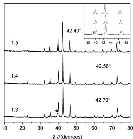
Fig. 3 The XRD patterns of the samples prepared from the precursors with different  $\text{Co}(\text{CH}_3\text{COO})_2$  and HMT molar ratios. The inset corresponds to the magnified portion. The asterisk denotes the  $\beta\text{-Mo}_2\text{C}$  impurity.
