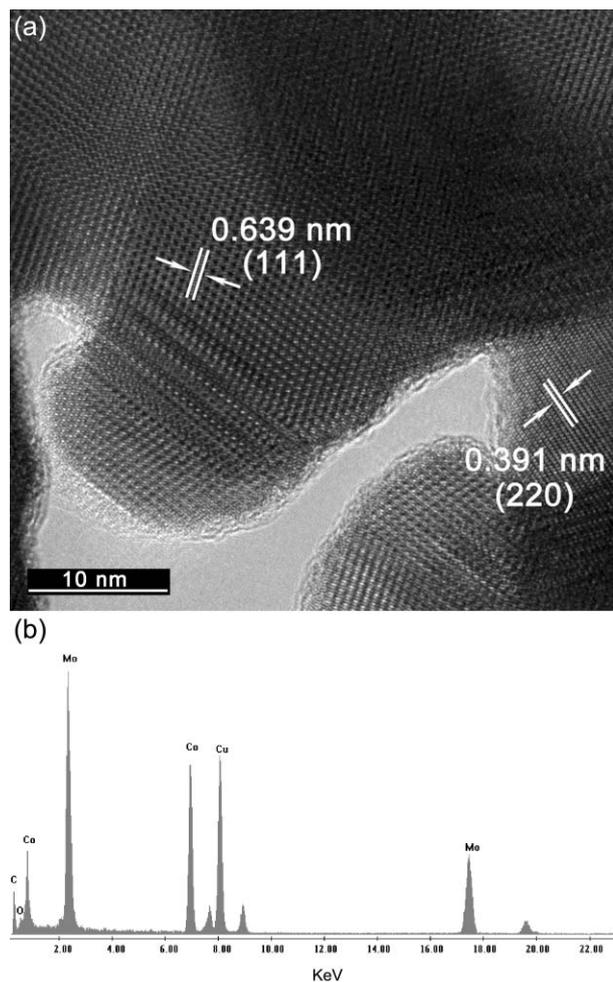
**Fig. 5** HRTEM micrograph (a) of as-prepared  $\text{Co}_3\text{Mo}_3\text{C}$  together with the EDX analysis (b) of this microregion.
