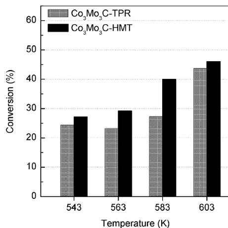
**Fig. 7** The 3-methylpyridine hydrodenitrogenation activities for Co<sub>3</sub>Mo<sub>3</sub>C catalysts prepared by the two methods.
