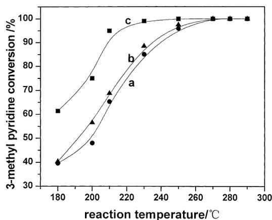
Fig. 4. The conversion and reaction temperature of 3-methyl pyridine HDN over various catalysts: (a)  $\text{NiMoN}_x/\gamma\text{-Al}_2\text{O}_3$  (5 wt.%; (b)  $\text{NiMoN}_x/\gamma\text{-Al}_2\text{O}_3$  (5 wt.%, 10 wt.%; (c)  $\text{NiMoN}_x/\gamma\text{-Al}_2\text{O}_3$  (5 wt.%, 15 wt.%). Conversion measured at 3.0 MPa and  $\text{WHSV} = 1.0 \text{ h}^{-1}$  for a reactant mixture containing 10% 3-methyl pyridine and 90% methyl cyclohexane.
