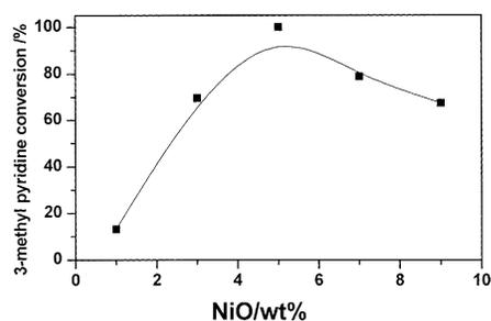
Fig. 5. Effect of the NiO loading on the conversion of NiMoN<sub>x</sub>/γ-Al<sub>2</sub>O<sub>3</sub> catalyst for HDN of 3-methyl pyridine. Conversion measured at 533 K, 3.0 MPa and WHSV = 1.0 h<sup>-1</sup> for a reactant mixture containing 10% 3-methyl pyridine and 90% methyl cyclohexane.
