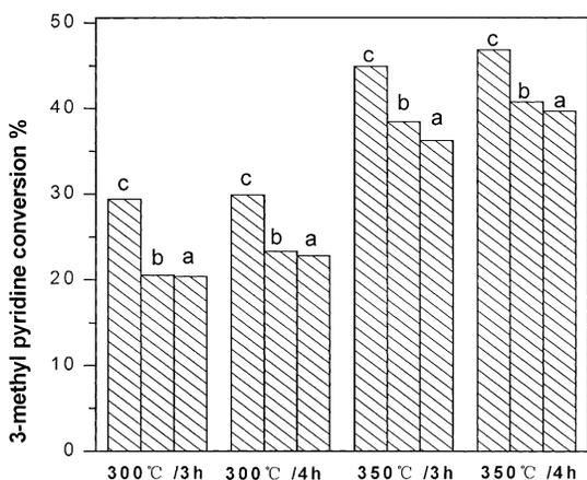
Fig. 3. Effect of reaction temperature and  $\text{MoO}_3$  loading ((a) 5 wt.%; (b) 10 wt.%; (c) 15 wt.%) on the conversion of  $\text{Mo}_2\text{N}/\gamma\text{-Al}_2\text{O}_3$  catalysts. Values measured at 3.0 MPa and  $\text{WHSV} = 1.0 \text{ h}^{-1}$  for a reactant mixture containing 10% 3-methyl pyridine and 90% methyl cyclohexane.
