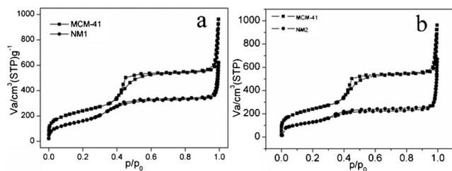
Fig. 2 Nitrogen adsorption/desorption isotherm of modified MCM-41 (a) NM1, (b) NM2.
