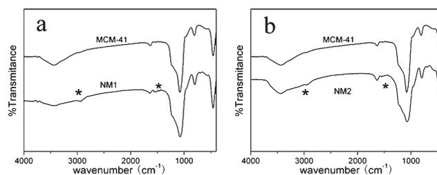
Fig. 3 FT-IR of modified MCM-41 (a) NM1, (b) NM2.
