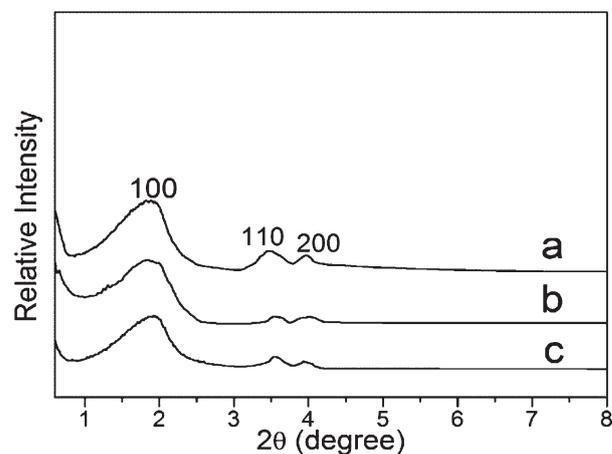
Fig. 1 The small angle XRD patterns of (a) MCM-41, (b) NM1, (c) NM2.
