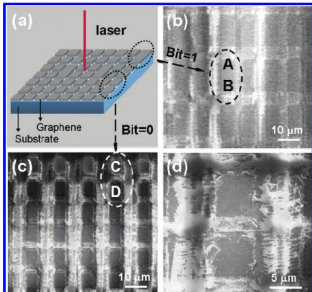
**FIGURE 3.** (a) Schematic illustration of the process of laser patterning of an array structure with different sizes of graphene pillars and cut channels on a continuous graphene film. (b) Typical SEM image for the array of unwritten rectangle bits (logical “1”). (c) Typical SEM image for the array of pairs of square bits all written with information (logical “0”). (d) Magnified SEM image of a pair of written bits. The thickness of the graphene film is approximately 40 nm.
