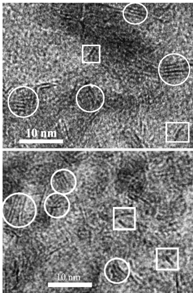
Fig. 6. HRTEM micrographs of the sulfided CoMo/ZA10 showing most multi-layer structured (circles) and some mono-layer structured (square) CoMoS clusters.
