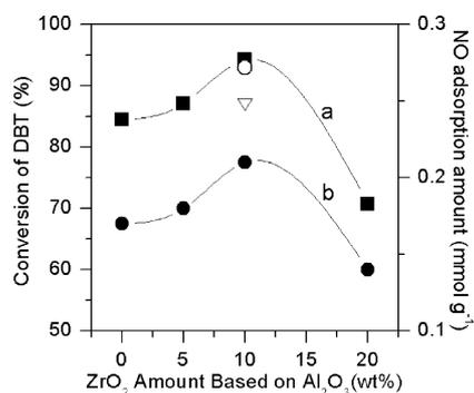
Fig. 4. (a) DBT HDS activities and (b) NO adsorption amounts of sulfided CoMo/ZA as a function of  $ZrO_2$  contents in the mixed supports based on  $Al_2O_3$ . The circle (○) and the inverted triangle (▽) are unrelated to the abscissa and denote the catalytic activities of KF757 in the same volume and weight as CoMo/ZA10 catalyst, respectively.
