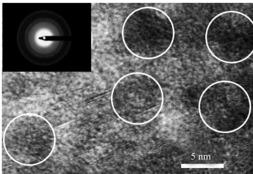
Fig. 3. HRTEM micrograph and SAED pattern (the inset) of ZA10. The circled fields are considered as  $ZrO_2$ .
