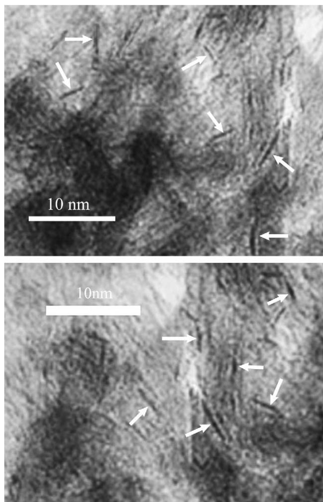
Fig. 5. HRTEM micrographs of the sulfided CoMo/Al showing only mono-layer structured CoMoS clusters.
