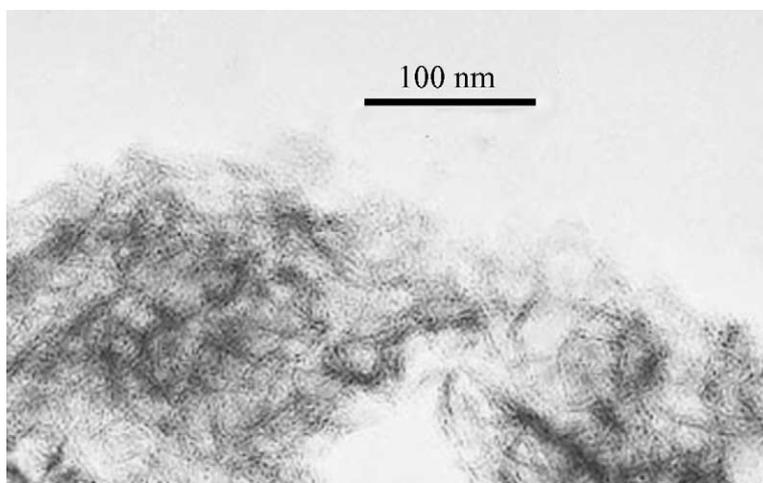
Fig. 2. TEM micrograph of ZA10. The black points mean  $ZrO_2$  particles.
