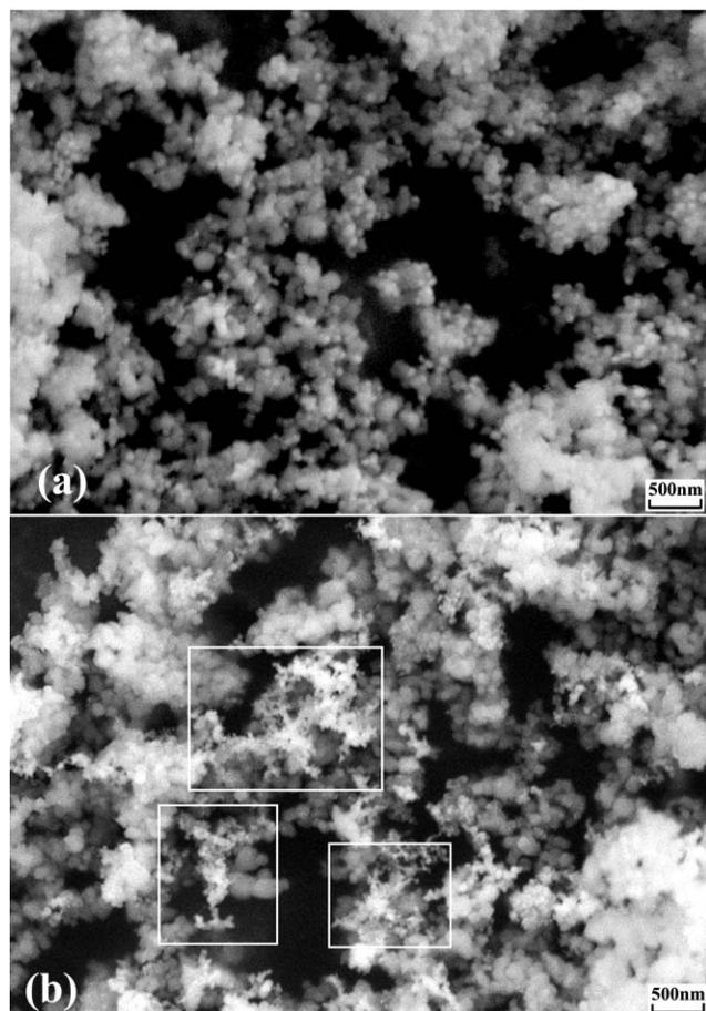
Fig. 2 SEM micrographs of (a) Ni-B(EN)/TiO<sub>2</sub> and (b) Ni-B(IR)/TiO<sub>2</sub>.
