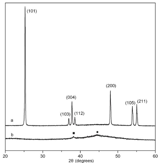
Fig. 1 XRD patterns of (a) Ni-B/TiO<sub>2</sub> and (b) bulk Ni-B.
