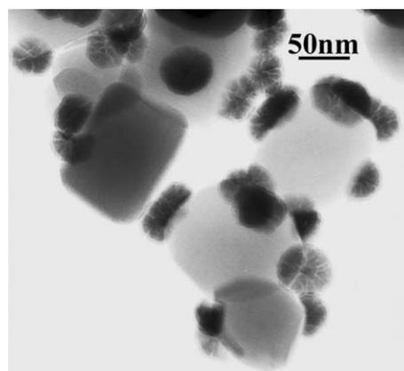
Fig. 3 TEM micrograph of Ni-B(EN)/TiO<sub>2</sub> catalyst.
