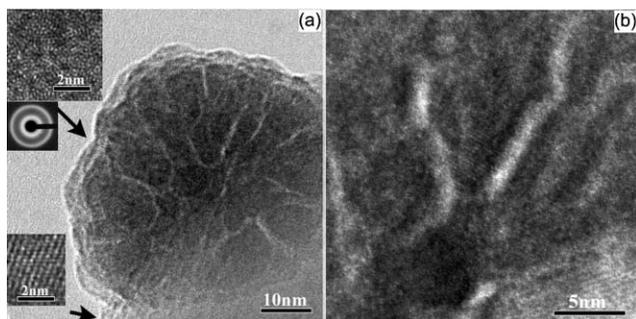
**Fig. 4** HRTEM micrographs of (a) Ni-B(EN)/TiO<sub>2</sub> catalyst and (b) the center of Ni-B particle. Insets: the corresponding SAED pattern of Ni-B and HRTEM images of Ni-B particle and TiO<sub>2</sub>.
