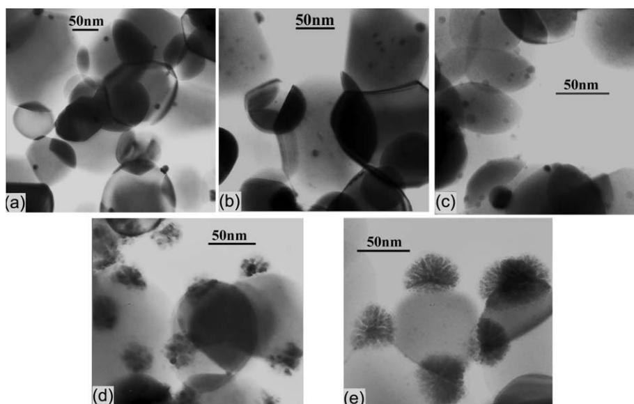
**Fig. 5** TEM micrographs of the intermediate Ni-B(EN)/TiO<sub>2</sub> samples at the different plating time (a) Ag/TiO<sub>2</sub>, (b) 8 min, (c) 12 min, (d) 18 min and (e) 28 min.
