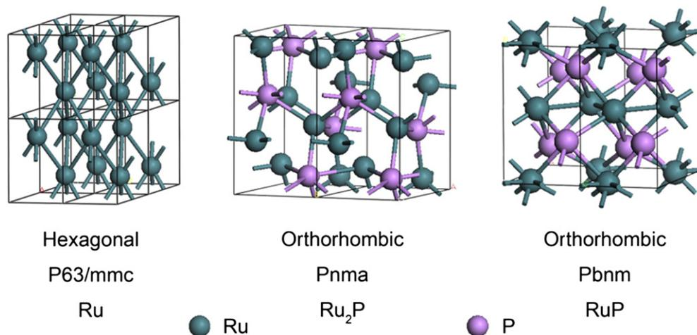
Fig. 1. The structure model of Ru, Ru<sub>2</sub>P, and RuP.
