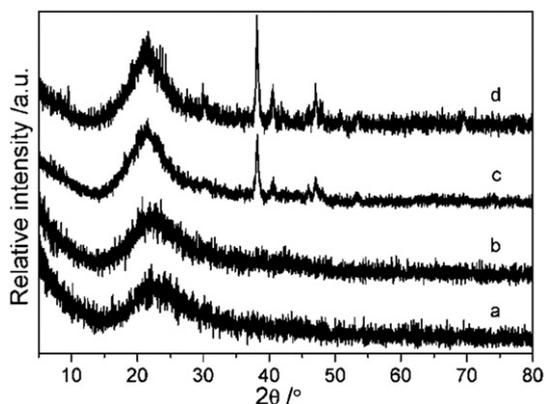
**Fig. 4.** The XRD patterns of the samples prepared from the supported precursors (MCM-41), which consist of  $\text{NaH}_2\text{PO}_2 \cdot \text{H}_2\text{O}$  and  $\text{RuCl}_3 \cdot 3\text{H}_2\text{O}$  in a molar ratio of 3.5 at different calcination temperatures for 1 h: (a) 573 K, (b) 623 K, (c) 673 K, (d) 773 K.
