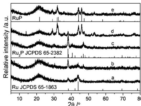
Fig. 3. The XRD patterns of the samples prepared from the supported precursors (MCM-41) at 673 K, which consist of NaH<sub>2</sub>PO<sub>2</sub> and RuCl<sub>3</sub>·3H<sub>2</sub>O with different molar ratios (NaH<sub>2</sub>PO<sub>2</sub>/RuCl<sub>3</sub>): (a) 1.75, (b) 2.00, (c) 3.50, (d) 5.0, (e) 5.75.
