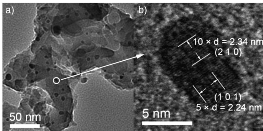
**Fig. 5.** The as-prepared  $\text{Ru}_2\text{P}/\text{MCM-41}$  catalysts with loading of 5 wt% treated at 673 K for 1 h in an Ar atmosphere: (a) TEM micrograph, (b) the magnified HRTEM image of the selected frame from image (a).
