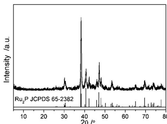
Fig. 2. The XRD pattern of the bulk Ru<sub>2</sub>P prepared from the precursors, which consist of NaH<sub>2</sub>PO<sub>2</sub>·H<sub>2</sub>O and RuCl<sub>3</sub>·3H<sub>2</sub>O in a molar ratio of 3.5.
