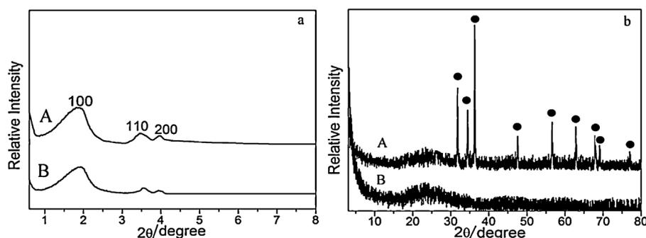
Fig. 1. (a) The small angle XRD patterns of MCM-41 and ZM; (b) the XRD patterns of MCM-41 and ZM ((a) A: MCM-41; B: ZM; (b) A: ZM, ●, the typical diffraction peaks of ZnO; B: MCM-41).
