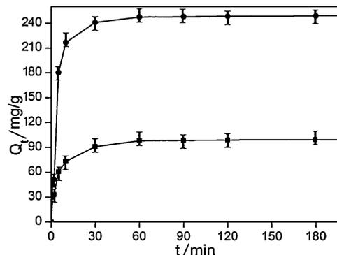
Fig. 4. Plot of Pb<sup>2+</sup> adsorption capacity Q<sub>t</sub> against contact time on ZM (adsorption conditions initial Pb<sup>2+</sup> concentration = (200 and 500) mg/L, adsorbent dose = 2 g/L, pH = 7, temperature = 298 K, contact time = 120 min (■, initial Pb<sup>2+</sup> concentration = 200 mg/L; ●, initial Pb<sup>2+</sup> concentration = 500 mg/L).
