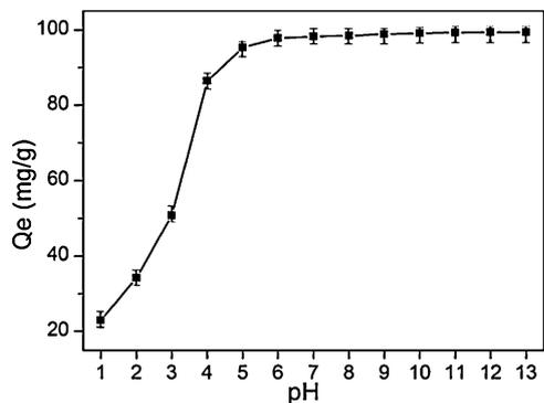
Fig. 2. Plot of % Pb<sup>2+</sup> removal against pH on ZM (adsorption conditions: initial Pb<sup>2+</sup> concentration = 200 mg/L, adsorbent dose = 2 g/L, contact time = 120 min, temperature = 298 K, pH = 1–13).
