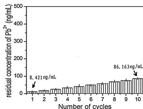
**Fig. 7.** Regenerated use of ZM for the removal of Pb<sup>2+</sup> (adsorption conditions: initial Pb<sup>2+</sup> concentration = 10 mg/L, adsorbent dose = 2 g/L, contact time = 120 min, pH = 7, temperature = 298 K) (1 mg/L = 1 μg/mol = 1000 ng/mL).
