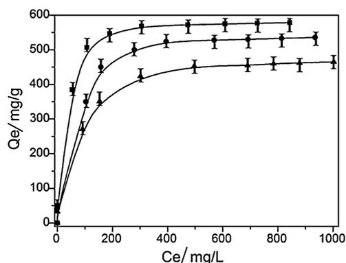
**Fig. 5.** Plot of  $Pb^{2+}$  amount adsorbed against different temperatures on ZM (adsorption conditions: adsorbent dose = 2 g/L, contact time = 120 min, pH = 7) (■,  $T = 323$  K; ●,  $T = 298$  K; ▲,  $T = 273$  K).
