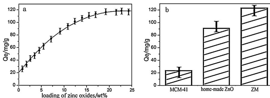
Fig. 3. (a) Plot of Pb<sup>2+</sup> adsorption amount at different concentration of functional group; (b) adsorption capacity of different adsorbents for Pb<sup>2+</sup> ((a) adsorption conditions: initial Pb<sup>2+</sup> concentration = 250 mg/L, adsorbent dose = 2 g/L, contact time = 120 min, pH = 7, temperature = 298 K).
