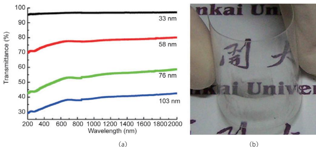
**Figure 3** (a) Optical transmittance spectra of films with different thicknesses on a quartz substrate; (b) a picture of a graphene-PEDOT film with a thickness of ~32 nm on a transparent PMMA substrate
