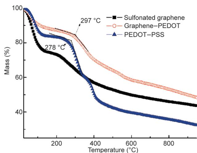
**Figure 4** TGA spectra of sulfonated graphene, graphene-PEDOT and PSS-PEDOT obtained with a heating rate of 5 °C/min from room temperature to 400 °C under N<sub>2</sub>
