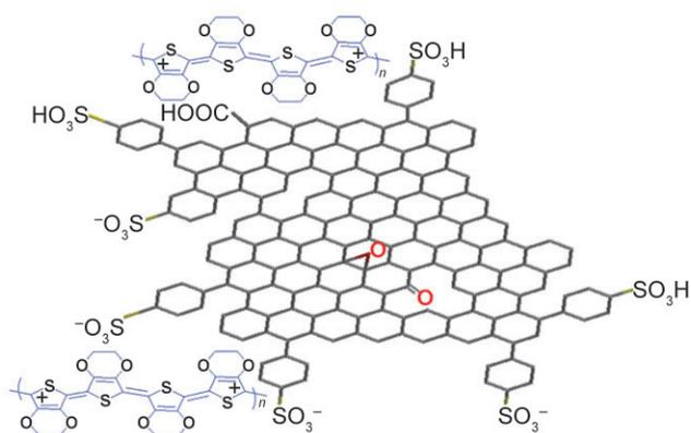
**Scheme 1** Schematic representation of part of the structure of graphene-PEDOT
