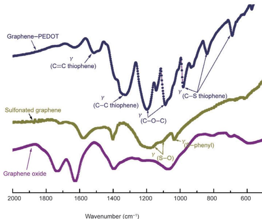
**Figure 1** FTIR spectra of graphene oxide, sulfonated graphene and graphene-PEDOT. The band at  $1513\text{ cm}^{-1}$  in the spectrum of graphene-PEDOT, arising from the C=C stretching vibration of the quinoidal structure originating from the thiophene ring, indicates the successful formation of the doped PEDOT
